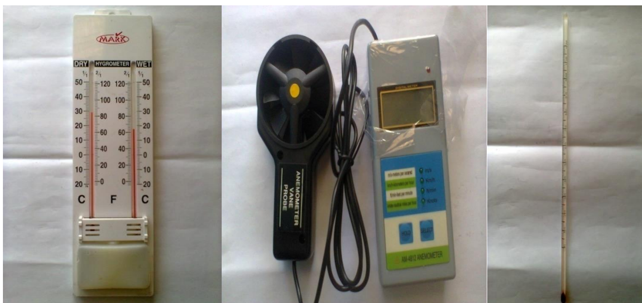
Plate I: Measuring instruments (Hygrometer, Anemometer and Thermometer)
